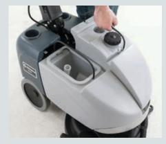
Easily remove the recovery and solution tanks to fill, drain and clean them away from the machine.
