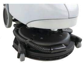
The SC351's rotating deck allows for both forward and backward scrubbing. Operators can push the machine forward in all directions like a "normal" scrubber. But, if the application requires, operators can quickly flip the machine up, triggering the deck to rotate completely for backward scrubbing performance. The scrub deck efficiently guides the wheels for superior edge cleaning.
