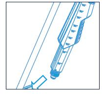
Use push buttons to attach or detach holder head.
