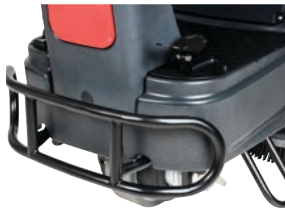
Standard front bumper protects the machine
