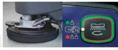
Optional splash guard keeps water in the path of the squeegee even at the fastest operation speeds.
