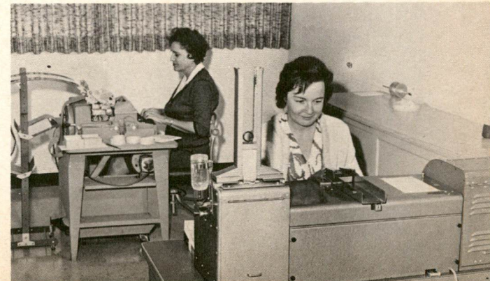
Betty Charle and Jane Stevenson process the new member applications received at World Headquarters. Mrs. Charle types receipts for the new member application fees. Mrs. Stevenson works at the automatic stencil typing machine which automatically types address stencils from Friden punch tapes.
